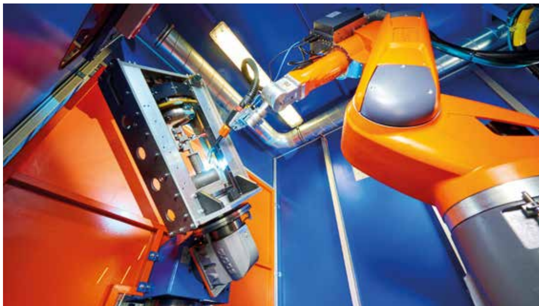
Compact robot cell to weld soft face hammers.
