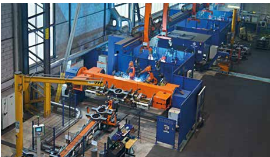
Concatenated robot line to weld drive axle bridges for utility vehicles at Voestalpine.
