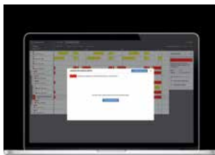
Visualisation: the cause of the alarm is displayed in the event of a fault in the plant. Unfiled errors can be quickly added.
