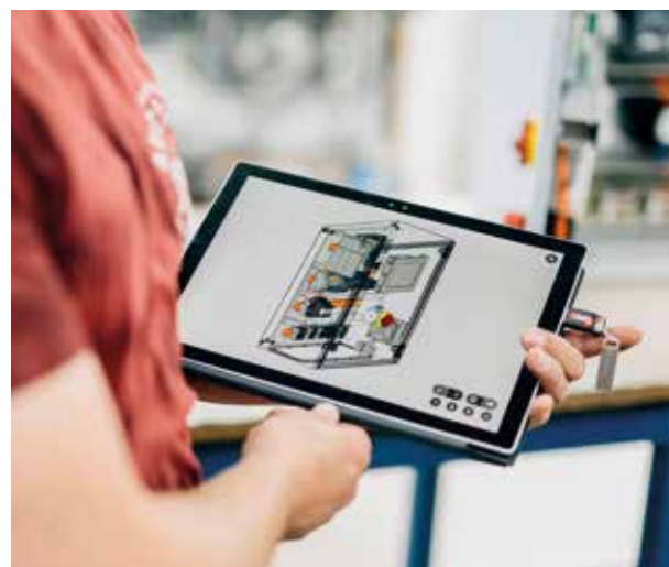
Digital twins of switching cabinets will now simplify the construction and assembly processes involved in building them.
