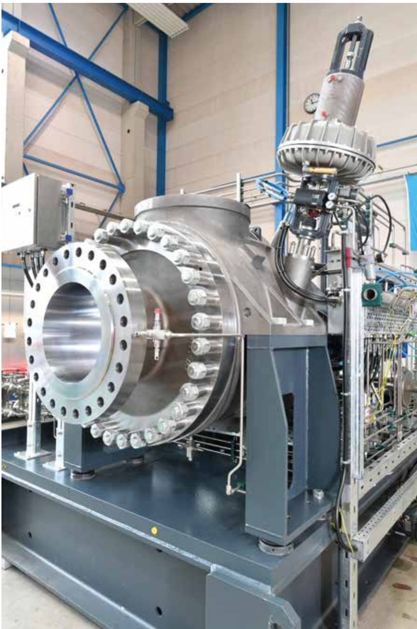
Expansion turbine for natural gas applications.
