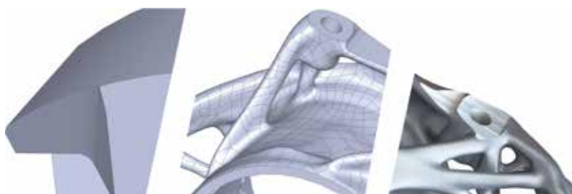
Step-by-step transition from a solid base body to an ideal lightweight structure for a wheel carrier.
