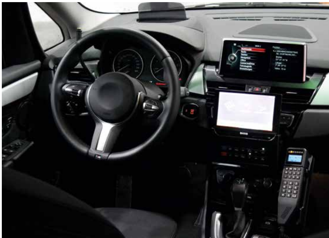
Trial installation of the new bracket to retrofit an emergency doctor's car with wireless and communications technology.
