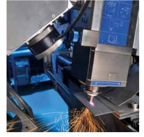
Laser cutting with tracking heat treatment laser. Local heat treatment can improve the crash properties of components by imprinting softer zones.
