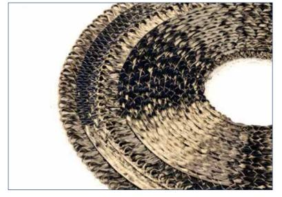
Technical embroidering machines allow radial and axial design of fibres according the flux process that has been defined in the component.
