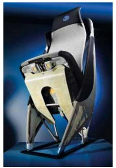
Lightweight truck seat with 20 kg weight saving at the top. The seat support made of glass fibre-reinforced plastics developed at the Fraunhofer ILT contributes to this.
