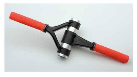
Compared to a hybrid component based on sheet steel, the hollow profile hybrid demonstrator has much greater dimensional stability, with better torsion stiffness and torsion strength.
