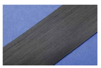
Tapes with endless fibres: the load-optimised arrangement of components helps to keep the overall weight down.
