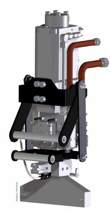
Wide-slot nozzle for wet compression moulding: this production method is suitable for series production of fibre-reinforced structural components. The reactive mixture is applied to the fibre roving as a fluid film. This is done either using robotguided application, or directly within the tool.
