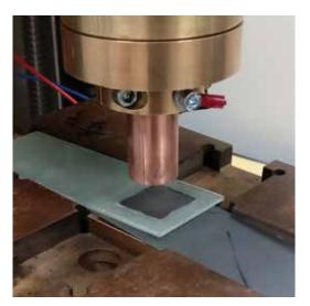
Welding an inserted hybrid test piece on a capacitor discharge welding system.
