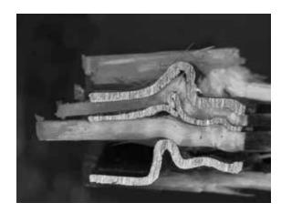
The situation that InHyb is trying to prevent: the bolt has deformed the metal sheet and damaged the GFRP material.
