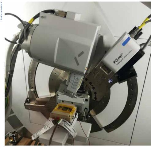
This equipment can be used to test the internal stress at different sample temperatures.
