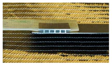
A finished welded hybrid test piece can be seen in cross-section.
