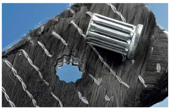
Laser beam-drilled CFC preform with internal threaded sleeve.
