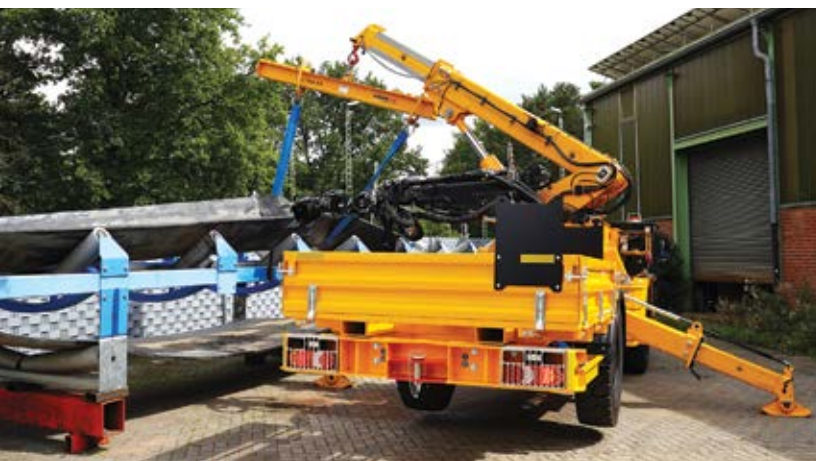
Using a Universa 50 base, Paus created an idler handler for the Oyu Tolgoi mine in Mongolia.
