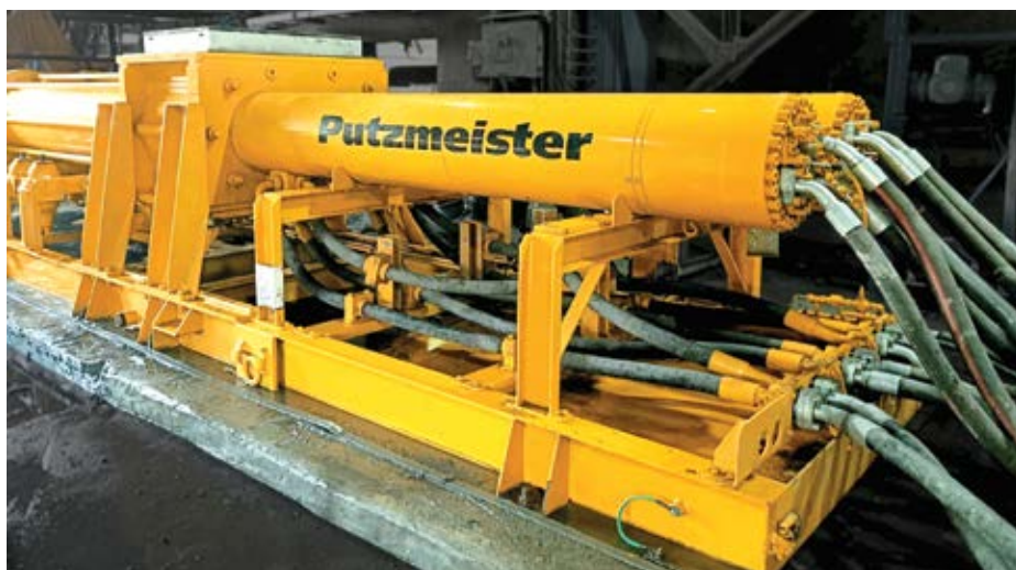
With 560-mm cylinders driven by a 2,500 kW hydraulic power unit, the HSP 25.200 HP is capable of conveying up to 240 m 3 /h of cementitious backfill.
