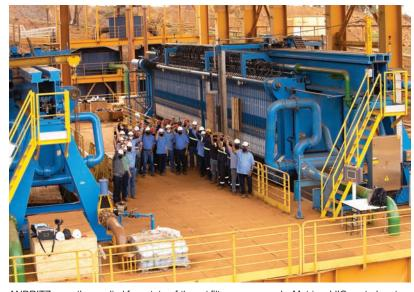
ANDRITZ recently supplied four state-of-the-art filter presses and a Metris addIQ control system for tailings dewatering to Brazilian iron-ore producer, Itaminas. (Photo: ANDRITZ)
