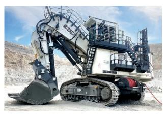
An R 9350 E electric excavator with the Liebherr cable reeler solution. (Photo: Liebherr)
