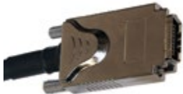
SFF-8470 connector (InfiniBand, CX4 or active optical cable)
