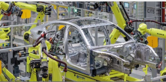
Robot guidance from AI° in the Porsche Leipzig body shop.
