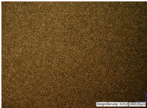
Figure 17b: Crater, but surface wetted with paint throughout (LABS-compliant), image taken with transmitted light
