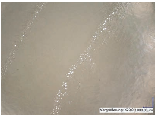
Figure 16a: LABS defects caused by paint wetting impairment substances dissolved from the O-ring, image with incident light
