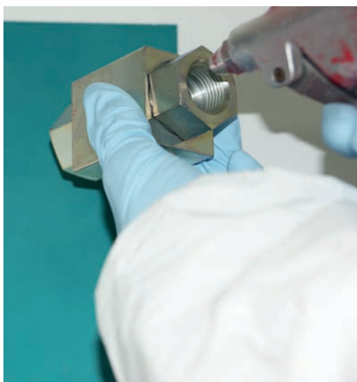
Figure 7 Blowing off an inner surface onto the test plate
